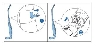
Insert the quick-mount screw into the screw hole on the upper body and tighten.
