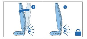
5. Take out the upper body, remove the quick-mount screw from the upper body, and insert the upper body into the lower body to ensure that the body is connected firmly.
