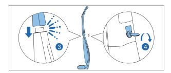
7. The battery is pre-installed. Do not remove unless necessary. If needed, loosen the screw and remove the battery.
