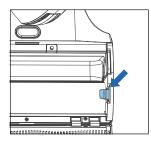
4. Push the lower body forward slightly and hear a "click", indicating that the lower body is locked in place.
