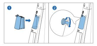
Insert the battery into the battery compartment of the lower body and tighten the screws to ensure that the battery is installed in place.
