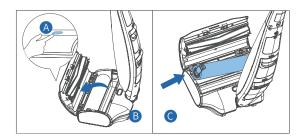
3. Push the cleaning roller back in and make sure that the snap-fit locks properly.
