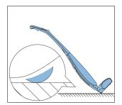
Note: If there is sand or other sharp objects on the floor, do not move the product with the wheels to avoid possible scratches.
