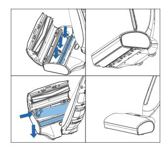
Note: Please make sure that all three snap-fits are locked when installing the wiper for proper use.Old cleaning rollers, brush rollers, and wipers are all plastic waste, so please dispose of them properly and recycle them according to local environmental laws and regulations.
