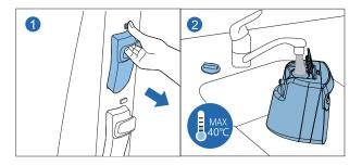
Note: Only use Hizero Cleaning Solution. Refer to the instructions of the Hizero Cleaning Solution. Add Hizero Cleaning Solution before adding clean water.
