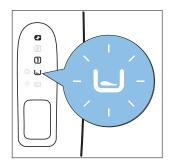
2.The indicator will flash red and the product will stop working when the dirty water tank is full. Please empty the dirty water tank (refer to Section 6.4 Empty the Dirty Water Tank) and re-start the product.
