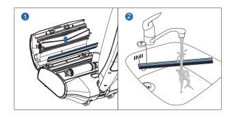
When the filter is clogged, wash the filter.
